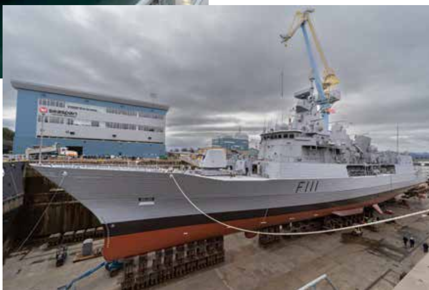
Below: HMNZS TE MANA with her new hull paint above and below, refreshing the anti-fouling and anti-corrosion capability of the hull. The white objects bolted to the hull are the sacrificial zinc anodes, to help minimise the electrolytic corrosion on the hull and other key underwater components.
